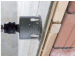
Diamond-ground tungsten carbide teeth, drop-shaped chip clearance slots.
